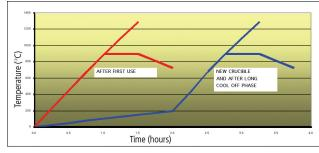
New crucibles and after long cool off phase — Heat empty crucible slowly to 200°C (390°F) to eliminate any moisture, then heat on full power to bright red heat. Crucibles for aluminium holding applications should be held at this temperature for 30 minutes to develop full glaze
