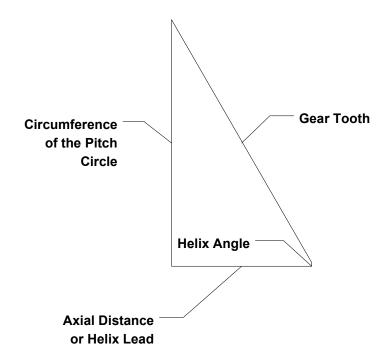
The left leg of the right triangle is the circumference on the Pitch Circle and is found by multiplying the Pitch Diameter by PI which is 3.14. The bottom leg of the triangle is the Helix Lead or the axial offset of the tooth for one full revolution of the gear. This distance can be calculated by dividing the Pitch Circle circumference by the Tangent of the Helix Angle.
