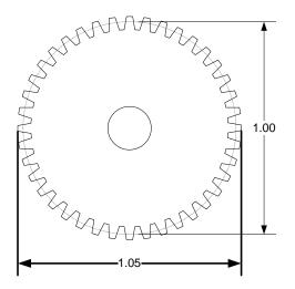
The circle with the dotted line in the gear to the left describes the pitch circle and its diameter is the pitch diameter, which is 1 inch. Since the gear has 40 teeth, this gear has a DP (diametral pitch) of 40.
