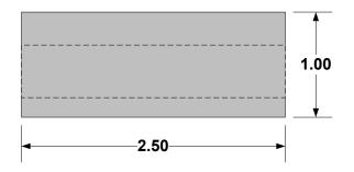
The spindle block is made from a piece of cold rolled steel I had on hand and was made to fit the milling vise on my 11" Logan Lathe. The size isn't critical. The gear blank will be positioned so that the teeth are cut in the top as it moves under the cutter.
